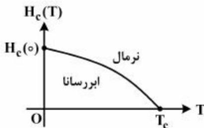
$$\alpha_0 T_c^{\gamma} = \gamma_0 + \gamma \mu_0 \left( \frac{H_c(0)}{T_c} \right)^{\gamma} \quad (1)$$
