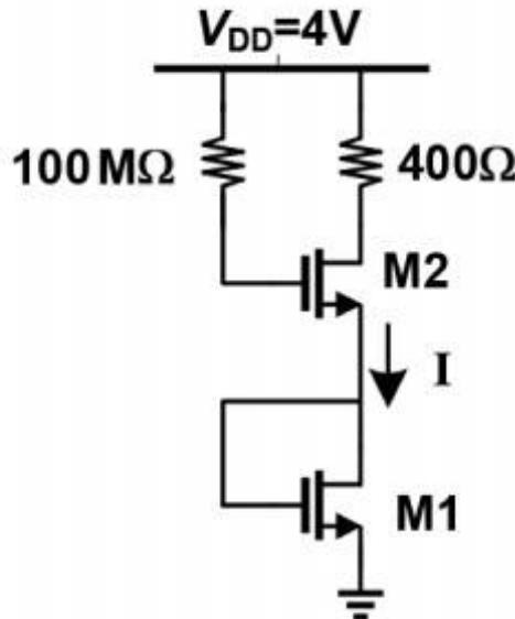
$$\mu_n C_{ox} = 5 \times 10^{-10} \frac{\mu\text{A}}{\text{V}^2} \quad V_T = 0.5\text{V}$$
