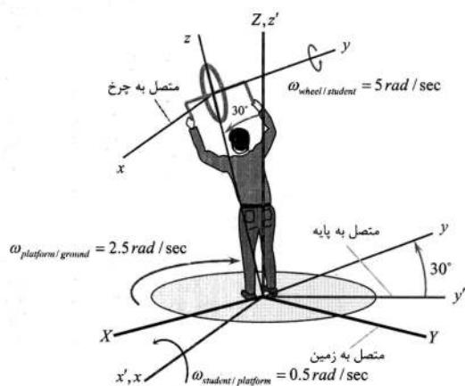
$$\vec{\omega}_{\text{wheel/ground}} = 0.5\vec{i} + 6.25\vec{j} - 2.165\vec{k} \frac{\text{rad}}{\text{s}} \quad (1)$$
